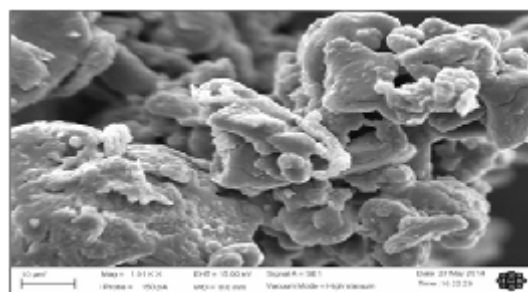
Fig. 9: SEM micrograph of SR \kappa C- g -PAA at a magnification of 1.01 Kx and the scale bar is 10 \mu\text{m}
