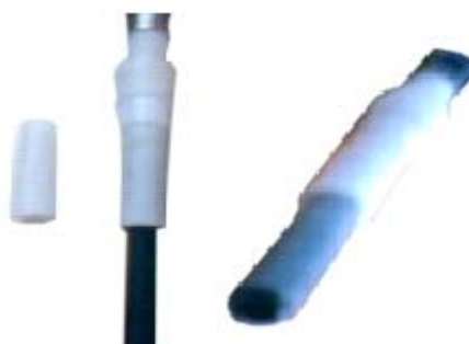
Fig. 4: The Teflon mold related to the graphite electrode, in both states of empty and filled with the paste related to membrane
