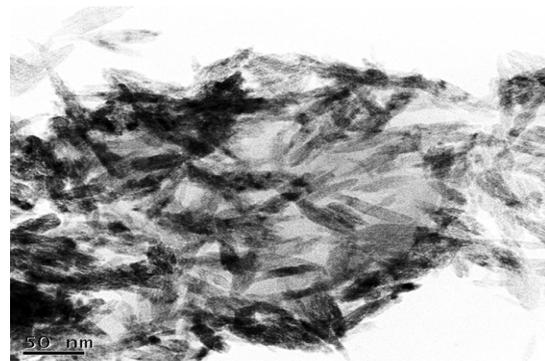
Fig. 5(a). HRTEM image of the synthesized CS-CuO nanocomposite
