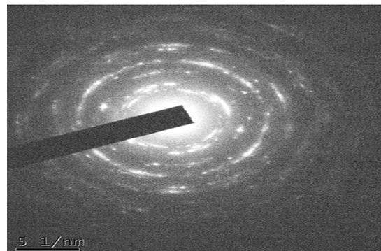
Fig. 5(b). SAED of the synthesized CS-CuO nanocomposite
