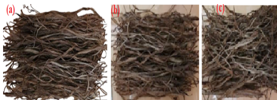
Fig. 1(a). Raw, (b) 5% NaOH modified (c) 10% NaOH modified Burmese silk orchid fibers
