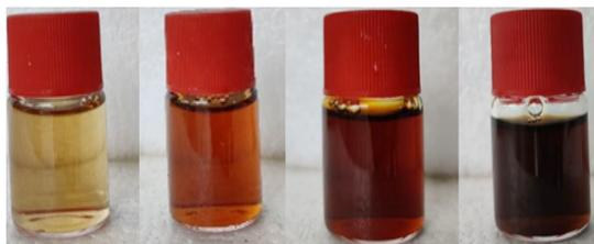
Fig. 1. Physical appearance (color change) of reaction media during synthesis of nanoparticle using *Lantana camera* leaf extract
