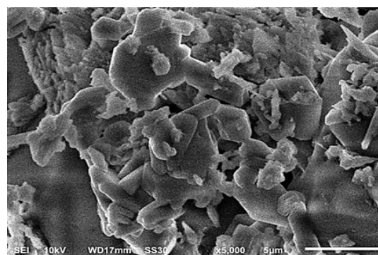
Fig. 3. SEM micrograph of calcium nitrite
