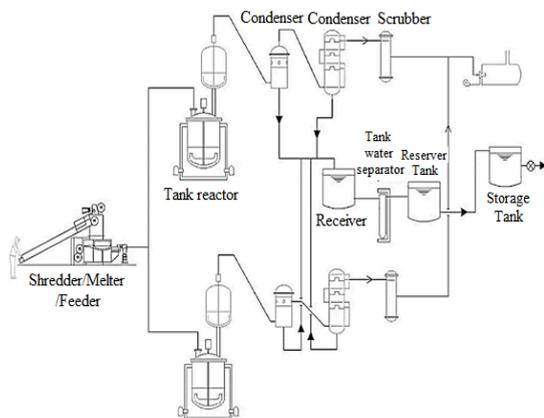
Fig. 1. Liquid Fuel Production Process (Source-Ref. no.-21)
