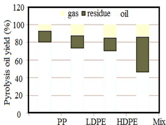
Fig. 5. The proportion of liquid fuel derived through pyrolysis from mixed plastics in municipal landfills, including PP, LDPE, and HDPE. (Source-Ref no. 18)
