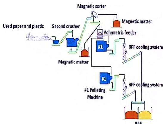
Fig. 2. RPF Production Process (Source-Ref. no. 21)
