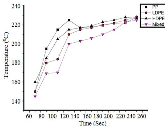
Fig. 3. The impact of varying reaction temperatures on the production of liquid fuel. (Source-Ref. no. 17)
