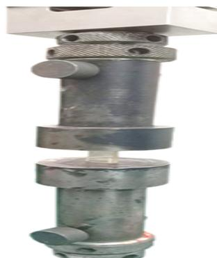
Fig. 4. The apparatus used to measure the compressive strength
