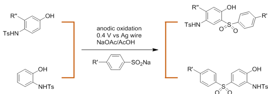
Scheme 1.8. Example of electrochemical anodic oxidation of aminophenols
