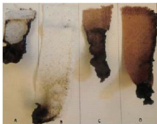
Fig. 6: Images of wool fabrics after the flammability test in acidic formic (A) untreated wool, (B) mordanted with 9% zirconium salt wool, (C) dyeing with madder wool (D) dyeing with madder and 9% zirconium salt wool
