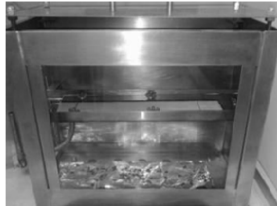
Fig. 2: Flame chamber used in this study with horizontal position for samples
