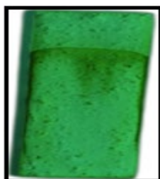
Fig. 6. TLC with derivatized chitosan, separation of borate complexed-mandelic acid
