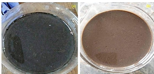
Fig. 3(a). Seed sludge (on day 0), and (b) AGS after 15 days of experimental work
