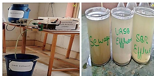
Fig. 1(a). A/O/A SBR reactor set up, and (b) Comparison of sewage, UASB effluent, and A/O/A SBR-treated effluent at the end of the study (Day 60)
