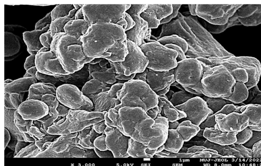
Fig. 4. Scanning electron microscopy (SEM) Images of Tamarind-2-Hydroxy-2-Methyl Butyric Acid (THMBA) resin
