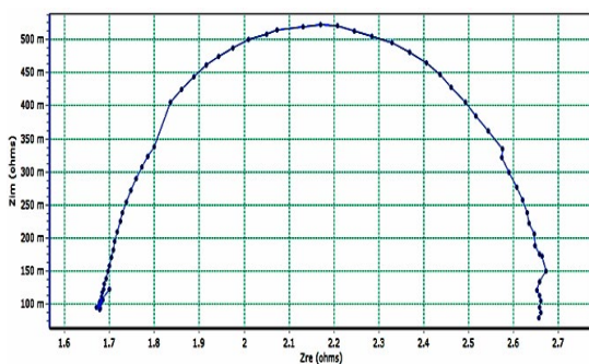
Fig. 6a. Nyquist plot in absence of optimum concentrations of rutin
