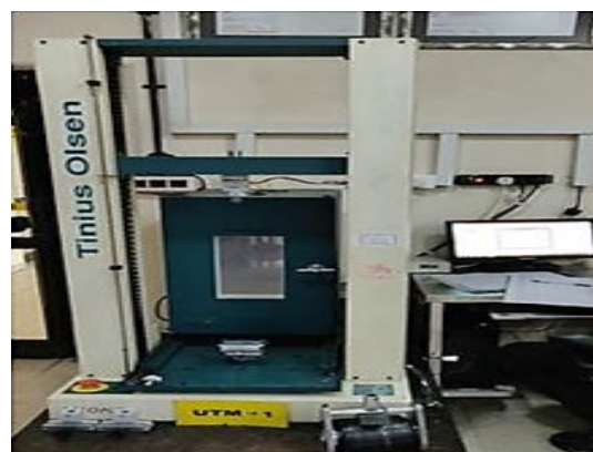
Fig. 4 a). Schematic diagram of peel strength method, b) A universal tensile testing machine
