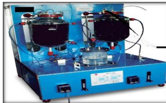
Fig. 1. Picture of the twin anaerobic digesters
