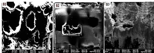
Fig. 3. SEM micrographs of polystyrene/FeS composite of various ratios of Sulphur. (A) B1-1:1 (B) B2- 1:5 (C) B3 1:8
