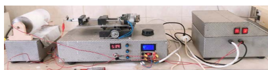
Fig. 3. Homemade electric spinning device
