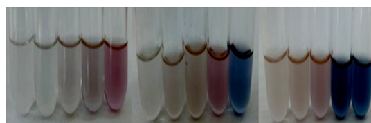
Fig. 5. Colloidal solution of Au nanoparticles at ratio volume of metal precursor : Extract of 6 : 14, 8 : 12, 10 : 10, 12 : 8 and 14 : 6 at metal precursor concentration of 0.4 mM (left), 0.6 mM (middle), and 0.8 mM (right)
