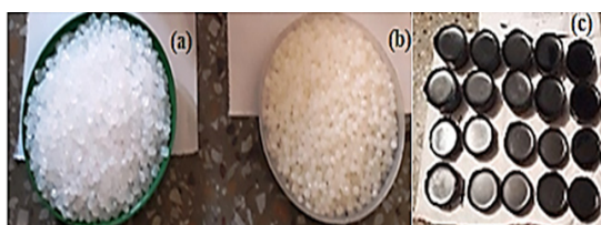
Fig. 1.(a). LDPE pellets (b) HDPE pellets (c) Modified Bitumen samples
