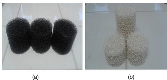
**Fig. 9. A blank of polyurethane foams 20 ppi (a), a sample of HPCM (b)**
