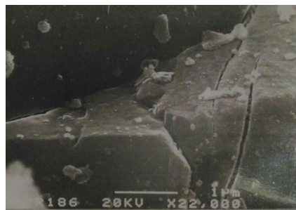
Fig. 7. Electron micrographs of alumina supported (\text{NH}_4)_2\text{Pt}(\text{ox})_2 \cdot 2\text{H}_2\text{O} after heating at 400^\circ\text{C} for 4 hours
