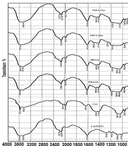
Fig. 1. FTIR spectra of \text{Li}_2\text{CO}_3 and catalysts
