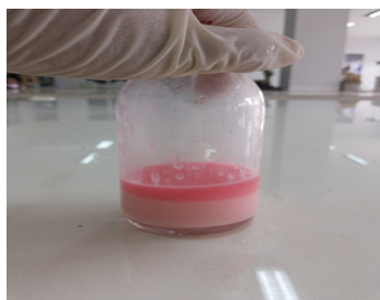
Fig. 1. A mixture of phosphatidylcholine and cholesterol in chloroform and SWEAF in a phosphate buffer solution pH 7.4 after sonication
