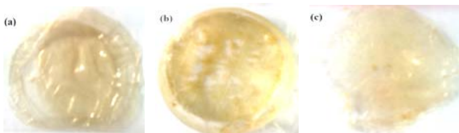
Fig. 3. Film forming of 1a chitosan (a), 1b chitosan (b) and Carboxymethyl chitosan (c)
