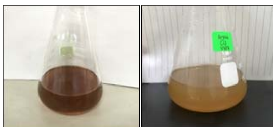
Fig. 1. Colour change of extract after addition of silver nitrate
