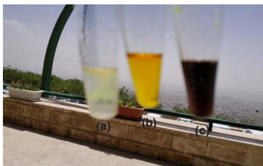
Fig. 1. a. Silver Nitrate Solution, b: Grapefruit's peel extract, c: Synthesis of Silver Nanoparticles
