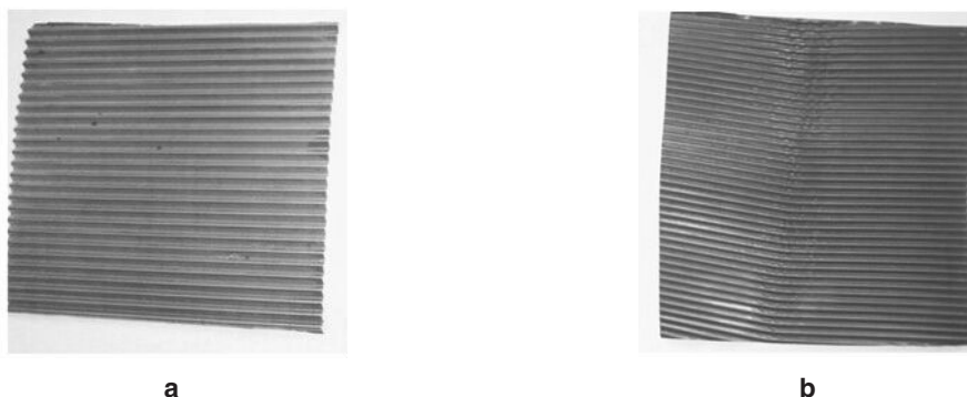
Fig. 1: The strips of corrugated foil: with channels of “direct” type (a), with channels of “chevron type” (b)
