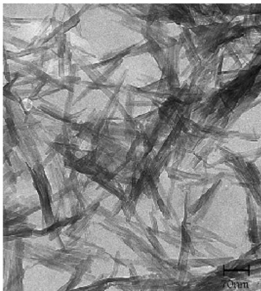
Fig. 3: The TEM image showing needle-like VSA particles of 15-20 nm in size
