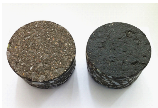
Fig. 1: Asphalt cores: the raw and processed impregnating composition
