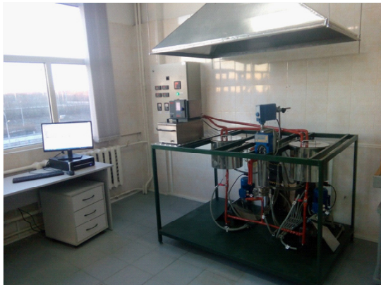
Fig. 1: Laboratory model of a flow reactor to produce a binder component
