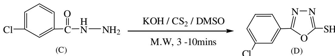
**Scheme 2: Synthesis of the ligand via microwave irradiation**
