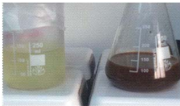
Fig. 1: Visual observation for the change in color of the reaction mixture after incubation at 50°C for 3 h
