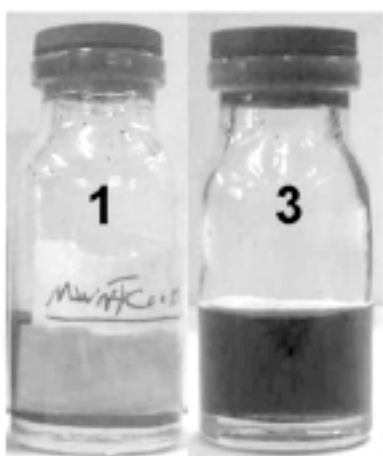
Fig. 6: The images of MWNT-COOH(1) and MWNT-benzoxazole(3) in DMF (1mg/8ml) after standing for 3 month
