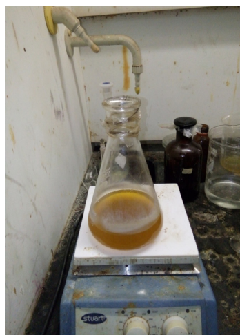
Fig. 1: The solution of \text{FeCl}_3 derived from the leaching process of HCl
