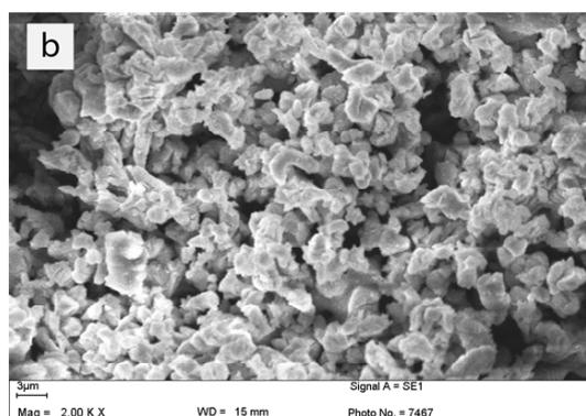
**Fig. 7: SEM micrographs of CaO powder after prepared from (a) chicken eggshells and (b) duck eggshells**
