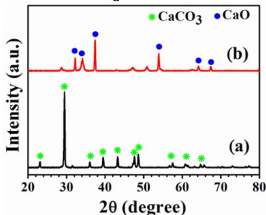
Fig. 3: XRD pattern of chicken eggshells (a) before calcined and (b) after calcined at 900°C
