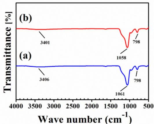
Fig. 2: FTIR spectrum of SiO<sub>2</sub> powder after prepared from (a) rice husk ash and (b) bagasse ash
