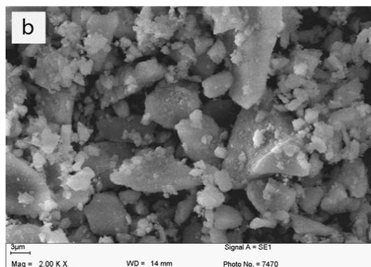
**Fig. 6: SEM micrographs of amorphous  $\text{SiO}_2$  powder after prepared from (a) rice husk ash and (b) bagasse ash**
