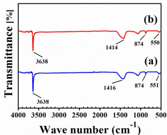
Fig. 5: FTIR spectrum of CaO powder after prepared from (a) chicken eggshells and (b) duck eggshells
