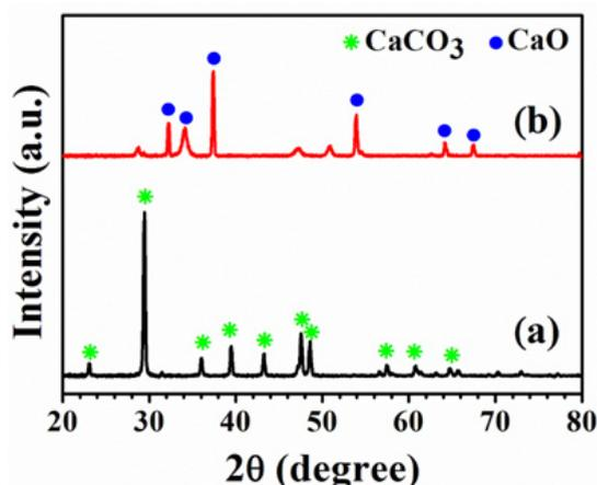
Fig. 4: XRD pattern of duck eggshells (a) before calcined and (b) after calcined at 900°C
