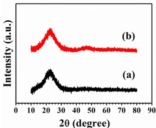
Fig. 1: XRD patterns of SiO<sub>2</sub> powder after prepared from (a) rice husk ash and (b) bagasse ash
