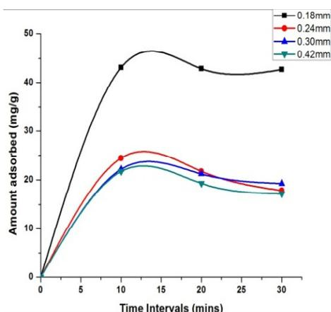
Fig. 3: Effect of Particle size
