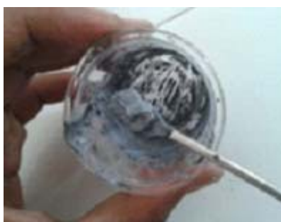
Fig. 1: Mixing of active carbon with TiO 2 in water medium
