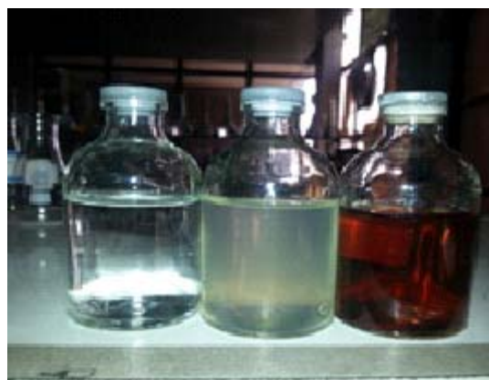
Fig . 1: (1) Silver nitrate ( \text{AgNO}_3 ) solution, (2) aqueous extract of Haliclona and (3) after the 4 h reduction of Silver nitrate
