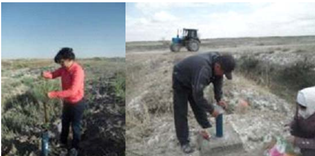
Fig. 1: Measurements of the level of occurrence and sampling of ground water for chemical analysis (2013)
