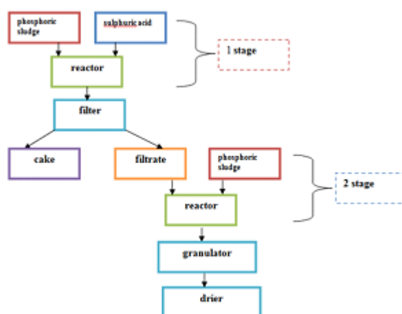
Fig. 1: Process flow scheme of acid decomposition of phosphorus sludge into superphosphate
