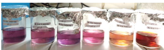
Fig. 5. Gold nanoparticle colloids synthesized with diabetic sugar without heating using microwave at pH 2, 4, 6, 8, 10, 12 at 0.6 mM Au precursor concentrations after several days
