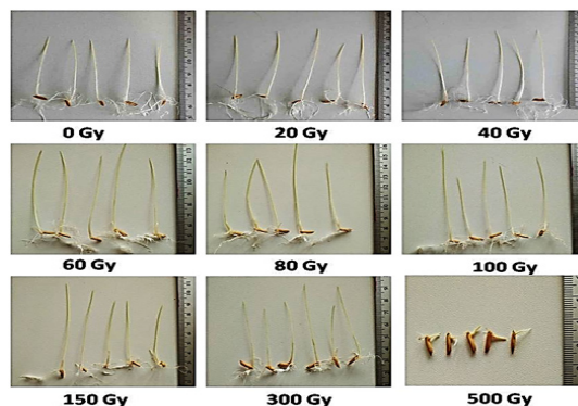
Fig. 4. Effect of gamma irradiation (20, 40, 60, 80, 100, 150, 300 and 500 Gy) on rice shoot-lengths of rice-seedlings (5 days old). 0 Gy means treating with no gamma irradiation
