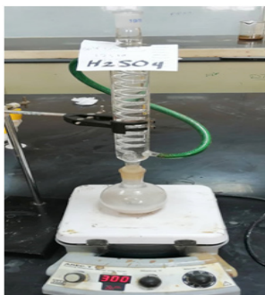
Fig. 3. Leaching system of calcined kaolin
