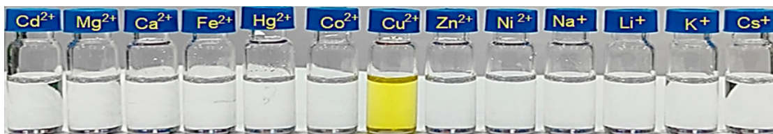
Fig. 5. Selectivity of compound-3 (100 \mu\text{M} ) for cupric ions compared to other metal ions
