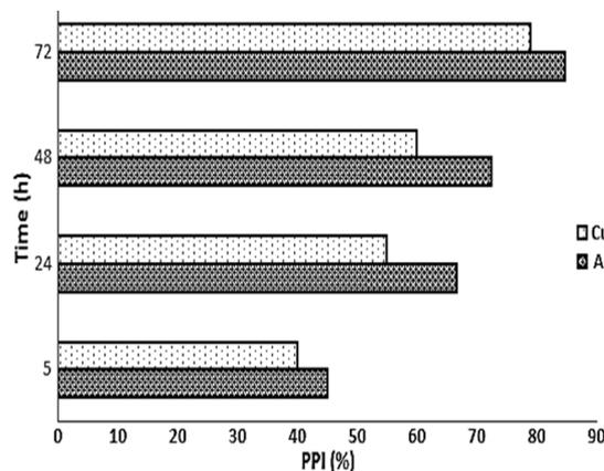
Fig. 12. Comparison of aluminum and copper corrosion rates in filtered biogas in this study
