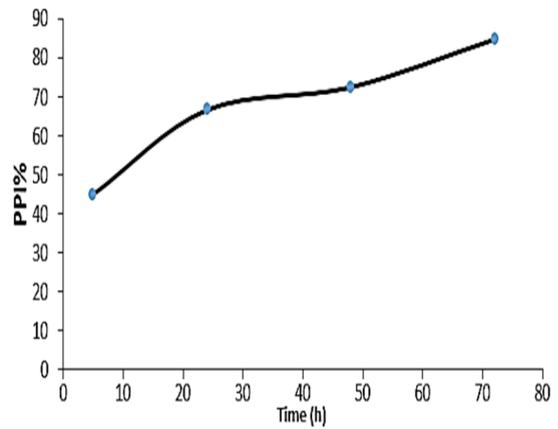
Fig. 11. Progression of the protective power induced in filtered biogas (copper case)
