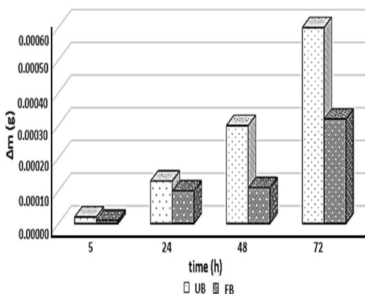
Fig. 5. Variation in copper mass loss over time in both unfiltered biogas (UB) and (FB)
