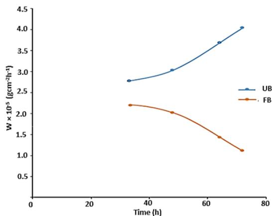
Fig. 7. Variation of the corrosion rate for copper
