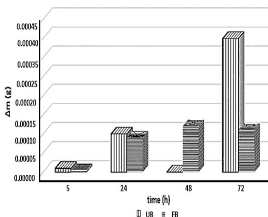
Fig. 4. Variation in aluminum mass loss over time in both unfiltered biogas (UB) and filtered biogas (FB)
