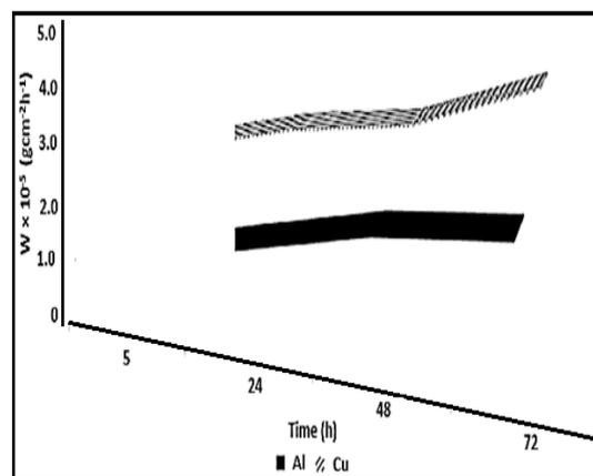
Fig. 8. Comparison of aluminum and copper corrosion rates in unfiltered biogas in this study
