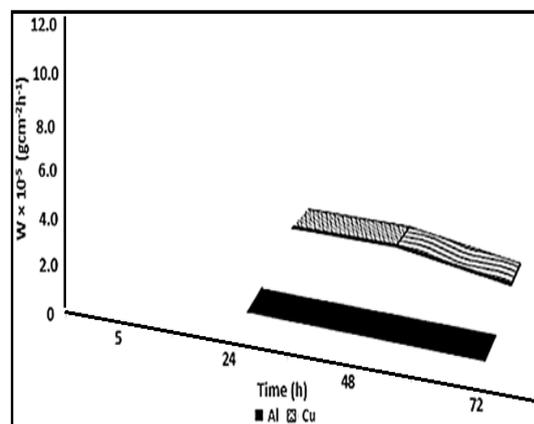
Fig. 9. Comparison of aluminum and copper corrosion rates in filtered biogas in this study
