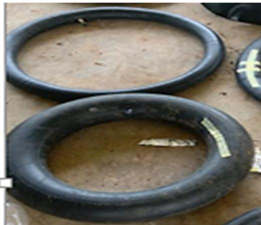
Fig. 3. The chambers filled with biogas and samples
