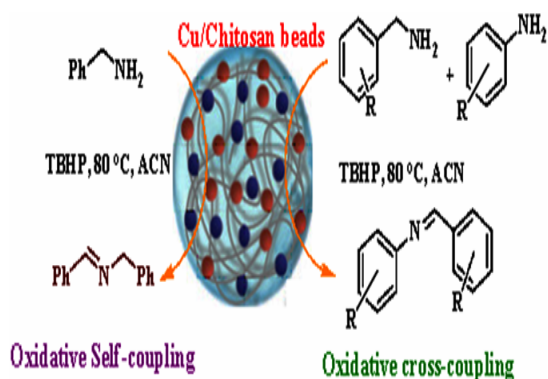
Scheme 3. Cu-coordinated chitosan beads as a catalyst in self-, cross-oxidative coupling of amines by TBHP for the selective synthesis of imines
