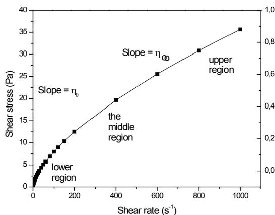
Fig. 1. Rheogram of a pseudoplast fluid with  $K=0.4 \text{ Pa}\cdot\text{s}^n$   $n=0.65$
