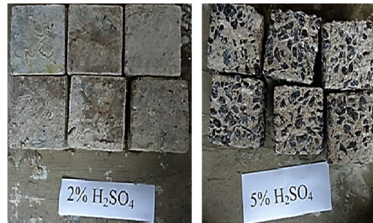
Fig. 5. A view of concrete cube specimens after being exposed to sulfuric acid
