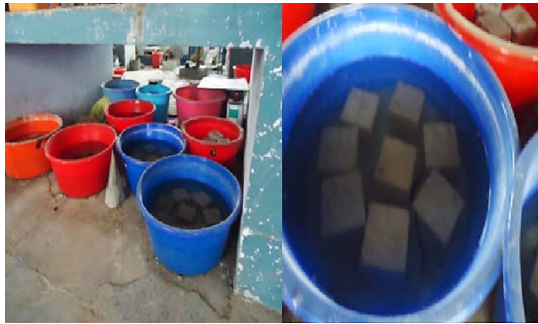
Fig. 2. A view of the test setup of cubes immersed in sulfuric acid solutions
