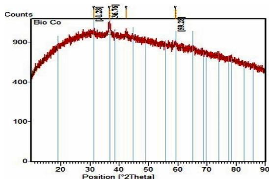
Fig. 3. XRD of biologically synthesized  $\text{Co}_3\text{O}_4$  NPs
