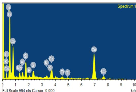
Fig. 2. EDX spectra of biologically synthesized  $\text{Co}_3\text{O}_4$  NPs
